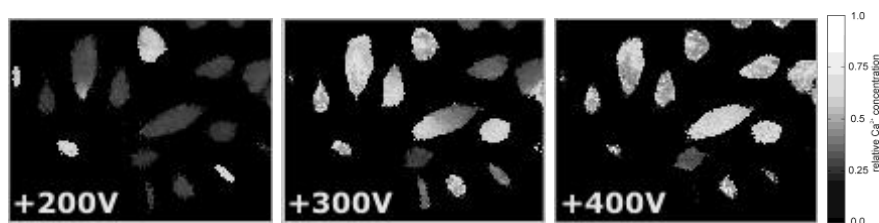
Figure 2: Cells stained with Fura-2AM and exposed to electric pulse with increasing amplitude.
